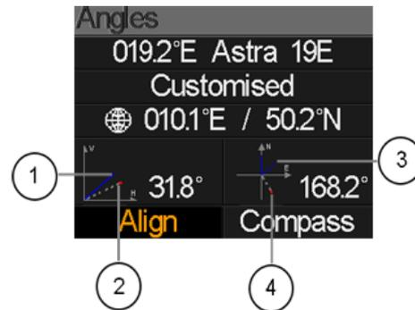
1. The current elevation simulated by meter
